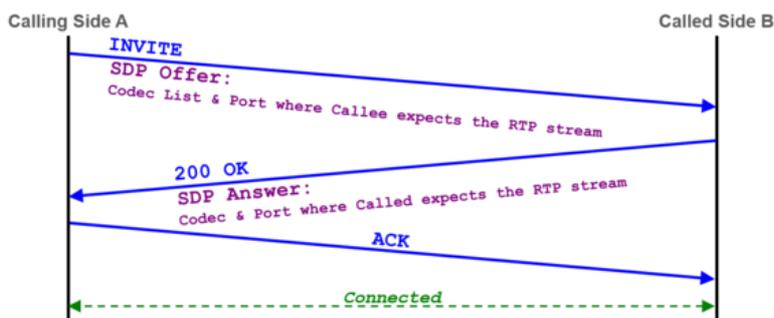
The following SDP properties and parameters are important for supporting customer problems:
