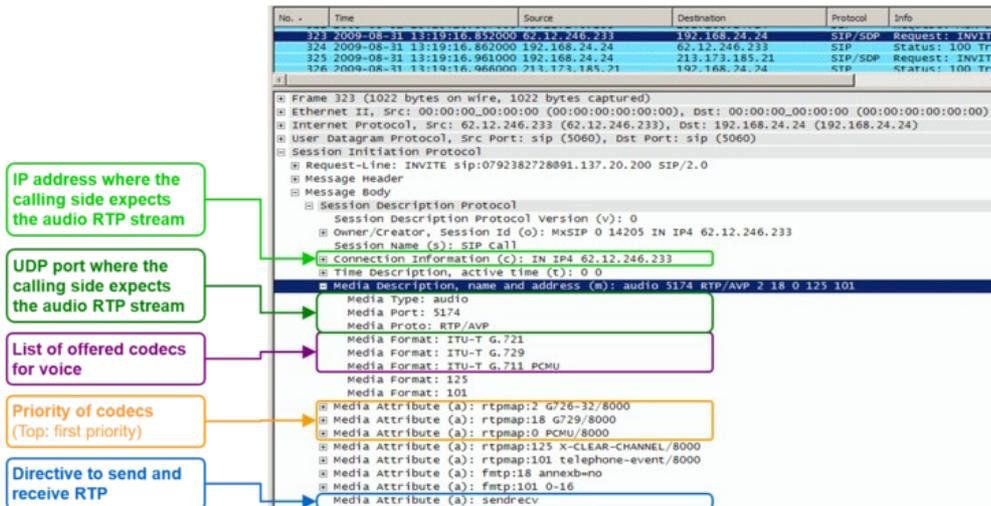
Example of a SDP offer for a Fax transfer with T.38 from the calling side A:
