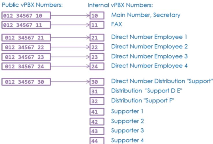
Based on this preparation the internal telephone numbers can be generated and the direct dialing in be configured.
